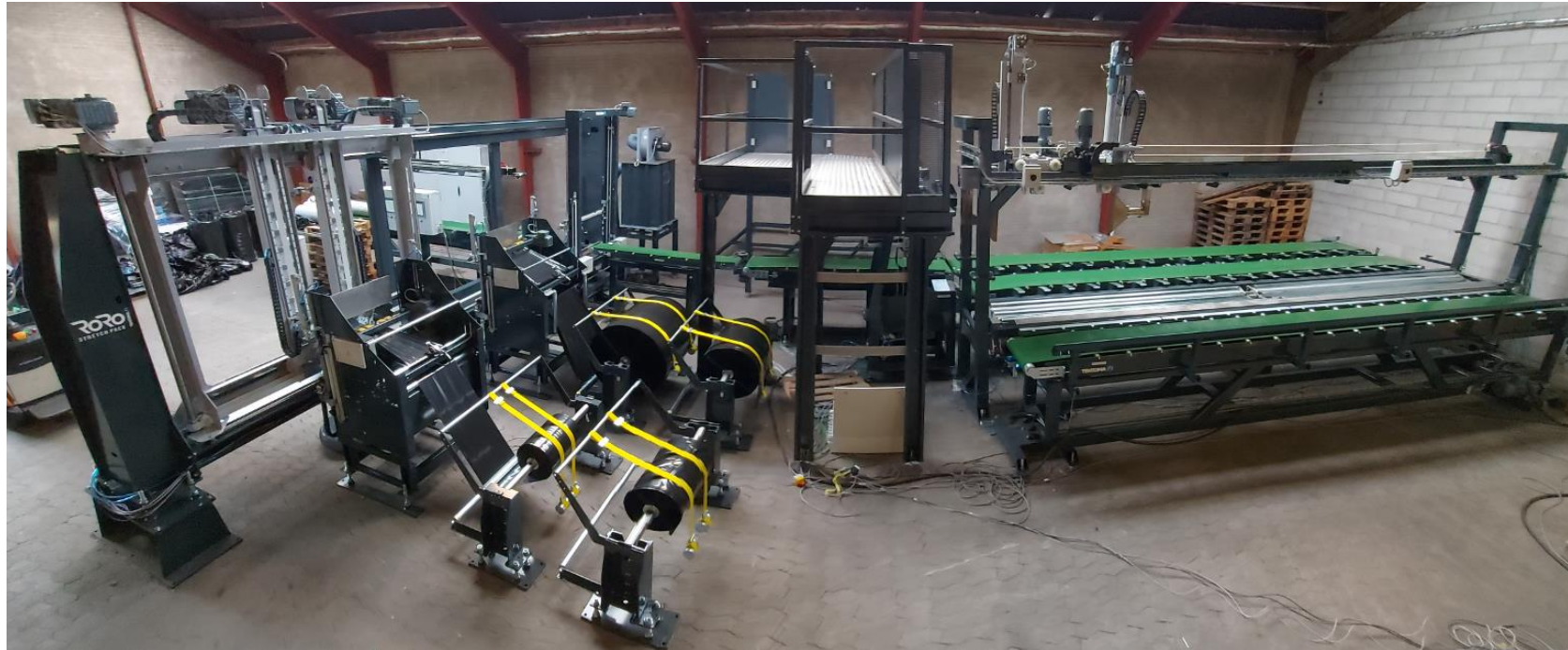
Geotextile inline solution Incl. plug applicator, heater and swing conveyors
