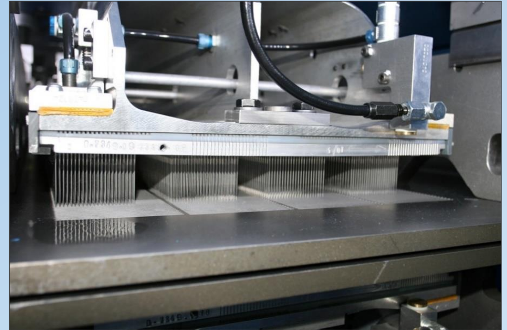
Intensive Needling Line, needling zone
