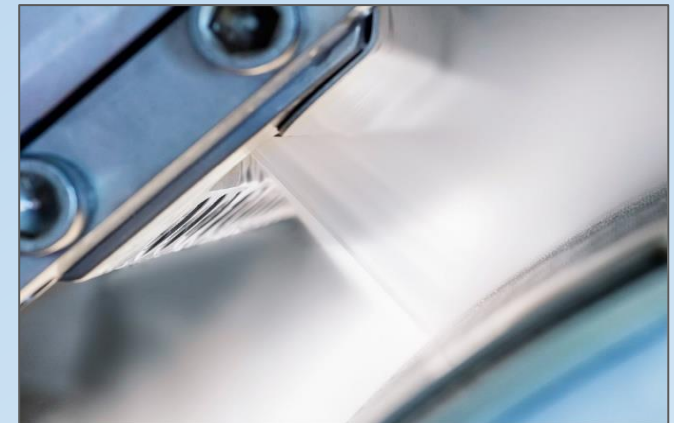
Water jet between beam and drum (Courtesy: Trützschler)
