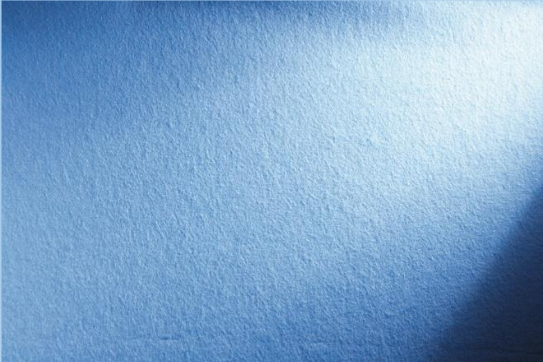
The needled product shows a homogeneous surface: intensely needled
