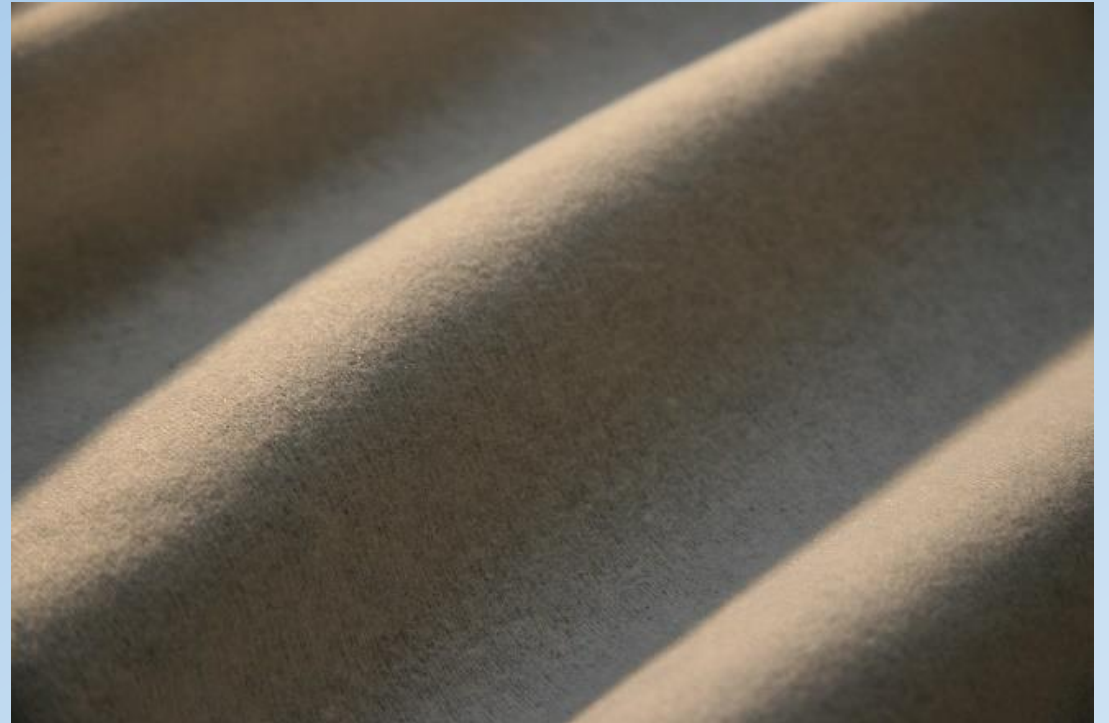
The hydroentangled product shows a homogeneous surface including the typical MD lines
